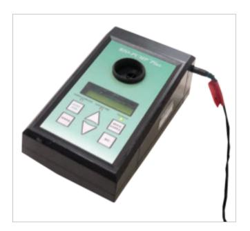
Step 1 Place the BIO-PUMP upright in the affected area, any height from 1.0m to 1.5m off the ground (e.g. on a table/
