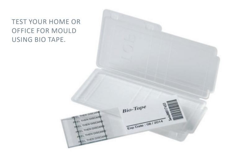
Surface Sampling is an effective way to allow lab technicians to analyse the source under a microscope in a remote location. The surface sample, has a film that is peeled off which exposes a slight sticky surface that collects particles off the test area when applied. This surface sample (sample slide), is then analysed under the microscope.
