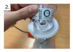
Firmly place the outttake hole of the Cassette into the head of the Air Pump. Hold the Pump in your hand at least 30cm away from any surface in the room.
