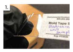
Put on gloves. Write a sample number and location description on the BioTape label. When ready to sample, hold by the label & peel off the plastic.
