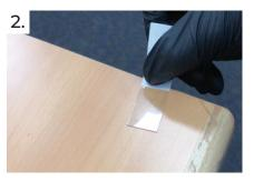
Try not to accidentally touch the adhesive (this could contaminate your sample). Press the exposed adhesive side onto the intended surface for 2 seconds and then release.
